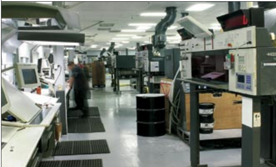
Williamson's Heidelberg presses equipped with the new JDF interface receive instructions from Prism, such as number of impressions and stock type.
